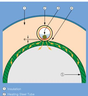
③ Special Skin-Effect Cable④ Thermal Junction⑤ Traced Pipe
